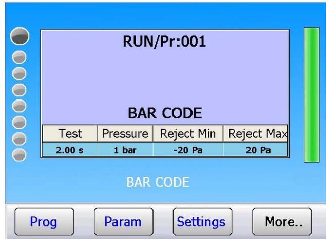
Then flash the code by using the bar code reader. The captured characters are displayed.
