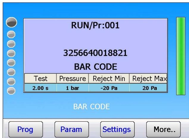
The code is recorded; the device is ready to run. At each reading of this code, the device will select the corresponding program and will start the test cycle if the "**AUTO START**" parameter is validated.
