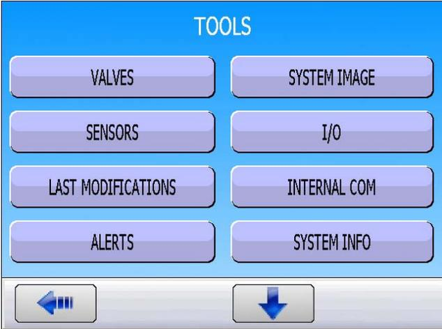
The list of the last parameters modifications is displayed on the screen; the list shows the current value and the old value.
