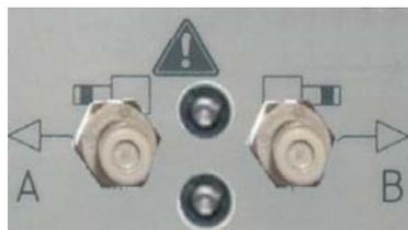
The automatic connectors A and B are dedicated for the pneumatic pilots of valves or to close simple fixtures.
