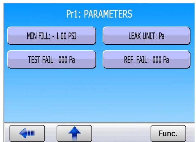
Change the **LEAK UNIT** from **Pa** to **cm3/min** or any other (flow unit) unit you would like to use.
