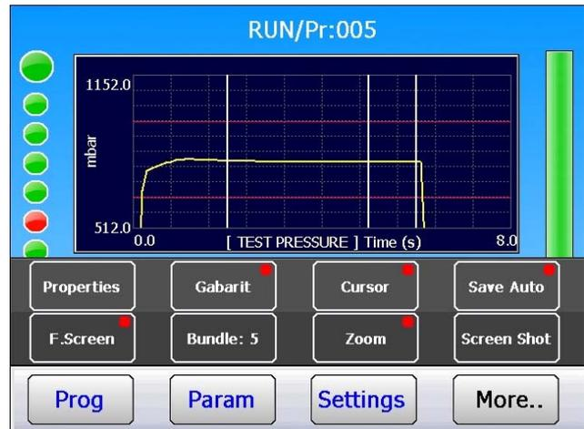
**Curve 2:** displays the leak curve.
