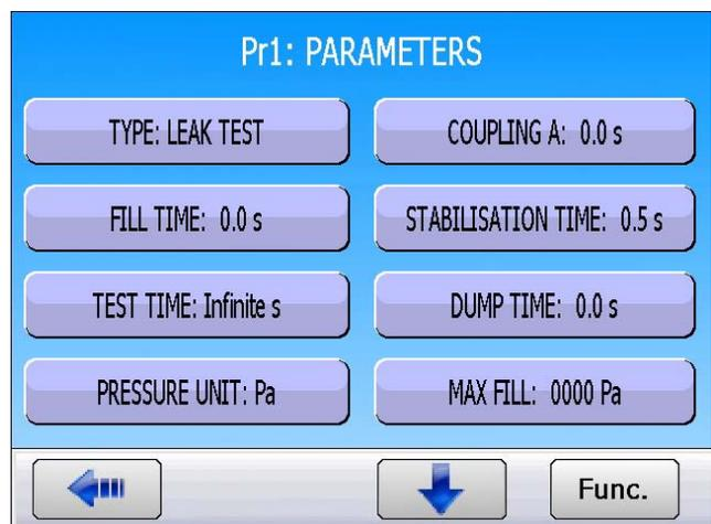
When all the parameters are entered, press on the "**START**" key. The instrument requests the regulator pressure to be set (in case of a mechanical regulator).
