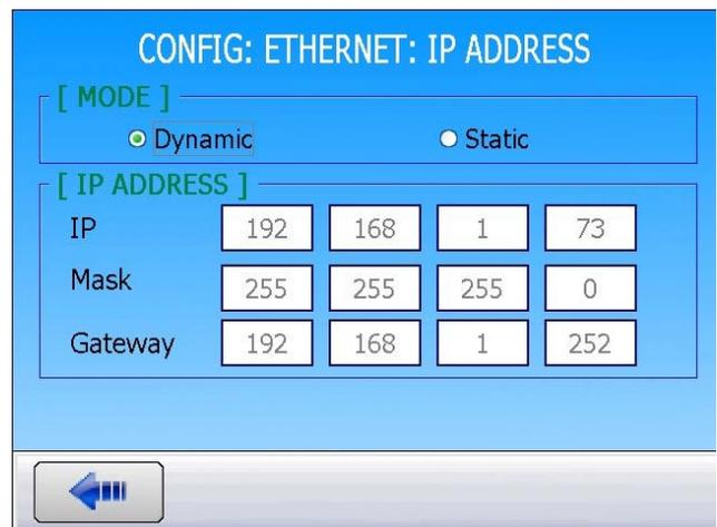
**Static** mode: the IP address must be entered manually.
