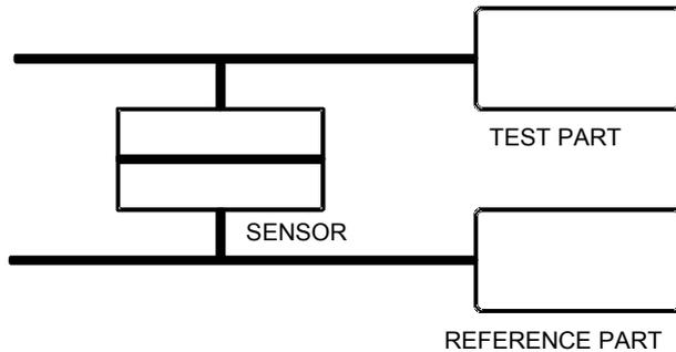
Measurement of a pressure variation between a test part and a reference part. The ideal measurement conditions are: part and reference part identical and identical **ATEQ** connections to both parts (identical lengths, diameters, and type of pipes). A measurement taken with a reference part saves time because the pressure equalization is more rapid. It is valid for parts which cannot be deformed and which mimic thermal and mechanical effects.
