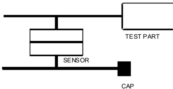
Measurement of a variation in pressure between a test part and a sealing connector on the reference side. A test without reference is not recommended unless parts with very small volumes are being tested. It is preferable always to have a certain volume on the reference side.
