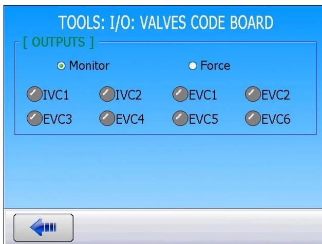
In **Monitor** mode: the user sees the I/O states, modified by the PLC or the device.
