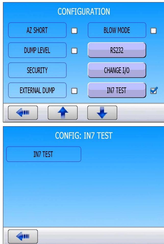
Then in the menu, click on the "IN7 TEST" button to enable the function.
