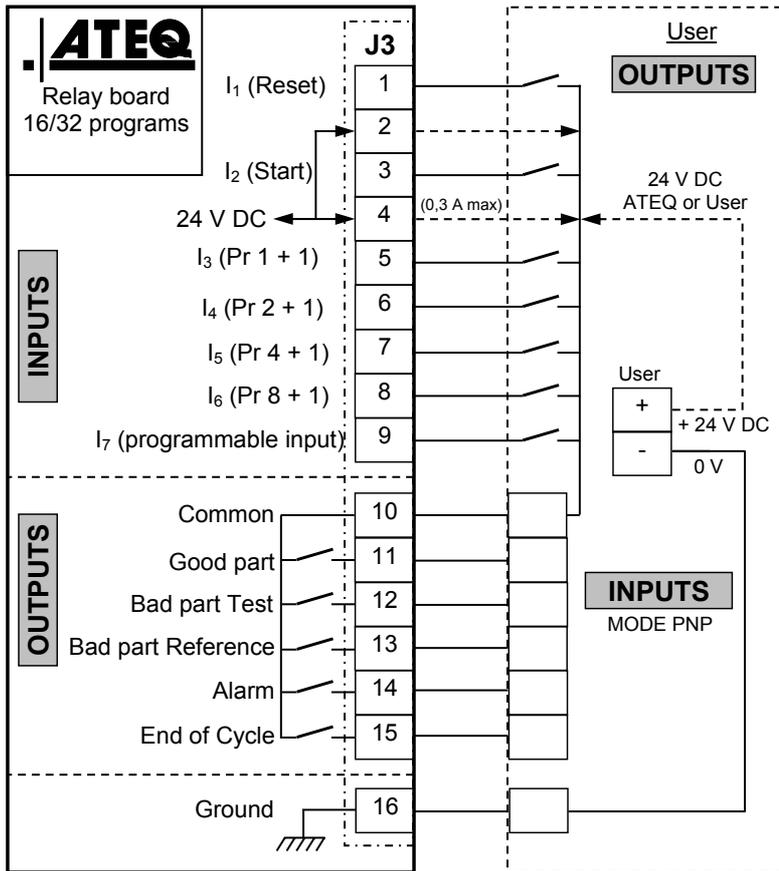
**Note:** The 24V power supply must be provided by the internal power supply of the ATEQ instrument (0,3A maximum) **OR** through an external power supply provided by the customer.
