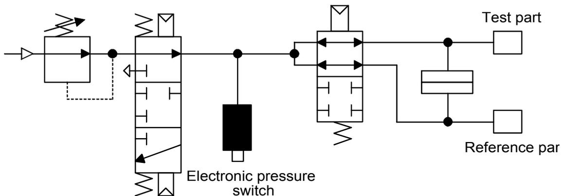
After filling the test and reference parts to the required pressure level, the instrument measures the differential pressure between the two volumes which are separated by the equalization valve.
