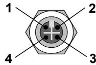
Used for connecting an intelligent remote control (female connector M12).
