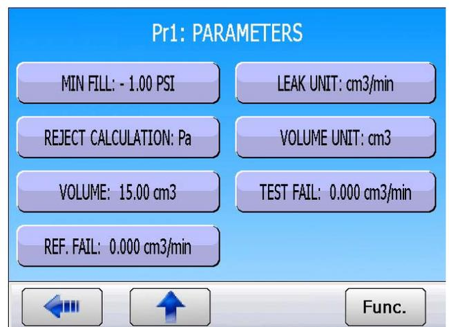
Enter the estimated value of the volume of the part to be tested, in the unit previously selected (cm3 in this example). The volume is the volume internal of the instrument + the volume of the tubing + volume of the part. The volume will be readjusted later.
