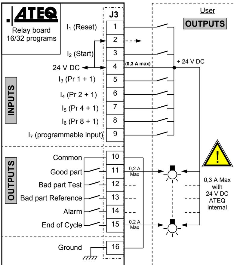
**Note:** The 24V power supply must be provided by the internal power supply of the ATEQ instrument (0,3A maximum) **OR** through an external power supply provided by the customer.
