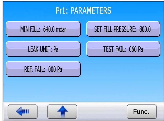
Press the parameter button to be modified, the keyboard appears. Enter the value then validate with **Enter**.
