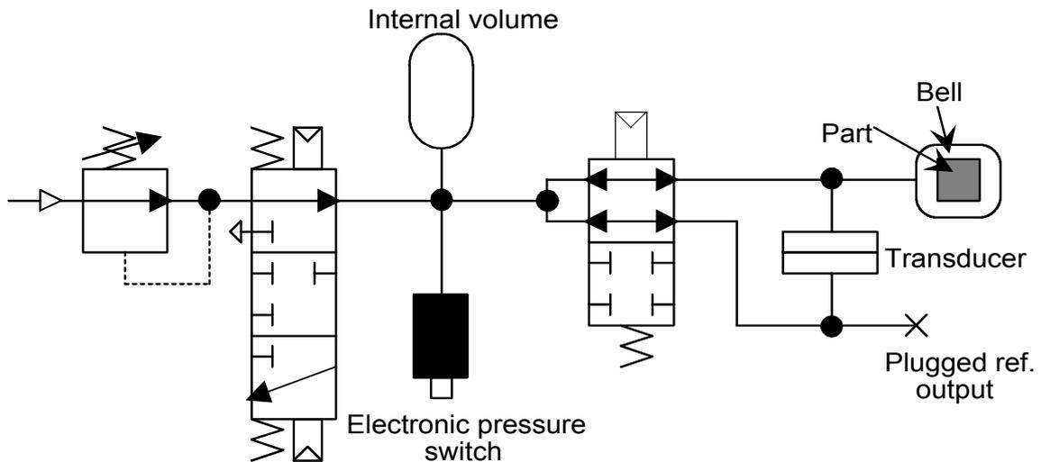
This test is intended for sealed parts which cannot be filled at the test pressure. They are put into the bell. The bell is pressurized by dumping air from an intermediary volume. The difference in the amount of air from a good to bad part can be measured. The pressure in the bell is controlled according to the formula:
