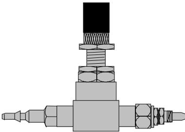
Needle valves are used to verify the leakage limits. These valves have an adjustable leak and depending on the model allow adjustments of between a few cm<sup>3</sup>/h to several l/min.
