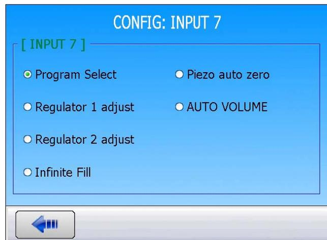
As well as the special maintenance cycles if that function is validated: "Regulator 1 adjust", "Regulator 2 adjust", "Leak sensor check", "Valve Auto-test", "Sensor status".
