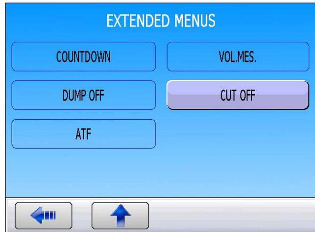
From the program **FUNCTIONS** menu, activate the **“CUT OFF”** function by checking it
