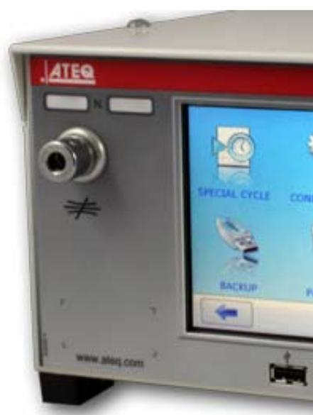
An optional Staubli quick disconnect is installed on the front panel of the instrument.
