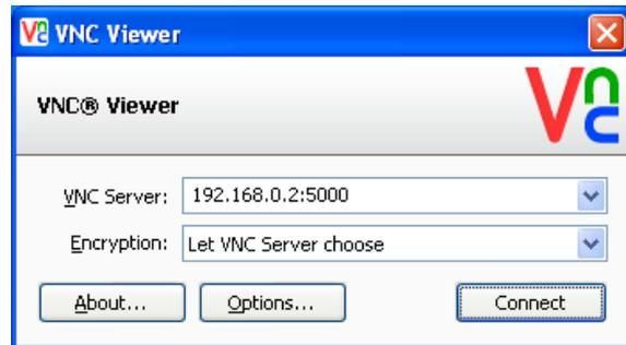
**Note:** in the case of IP address automatically assigned, you must know the ATEQ device one and enter it (with the port) in the field "**VNC Server**"
