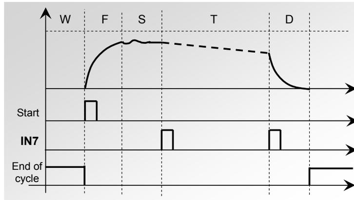
The jumps from "Stabilization" to "Test" and "Test" to "Dump" are validated by the input 7; the test time will be done by the user.
