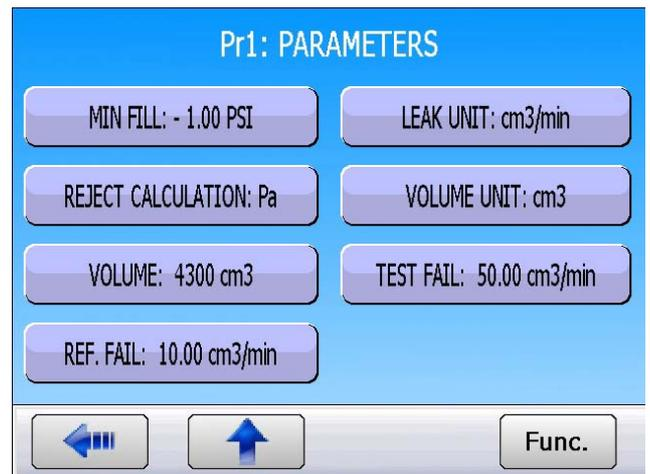
Enter the reject level for the leak test in the unit previously selected.
