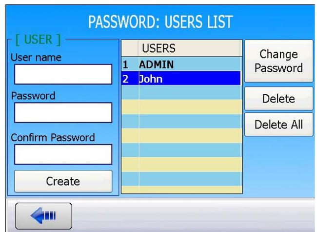
To delete the user, press **“DELETE”**. The instrument asks for confirmation.
