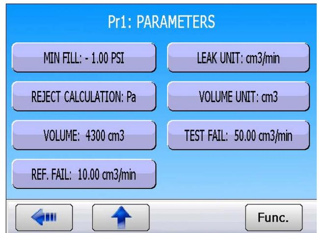
The relationship of the volume and the result is linear. If the displayed result is 10% higher than the calibrated leak value + Test result w/o leak, reduce the volume by 10%. Wait one minute between test cycles to ensure accurate results. Repeat as necessary.
