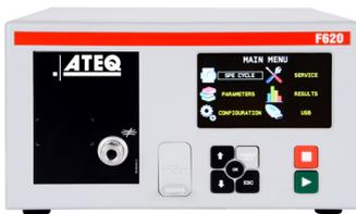
By far the most popular technology, differential pressure decay uses a reference volume to test your part. This helps compensate for any ambient pressure or temperature variations as they occur on both parts simultaneously. Only a leak on the test part will result in a movement of our transducer's membrane.
