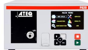
By far the most popular technology, differential pressure decay uses a reference volume to test your part. This helps compensate for any ambient pressure or temperature variations as they occur on both parts simultaneously. Only a leak on the test part will result in a movement of our transducer's membrane.
